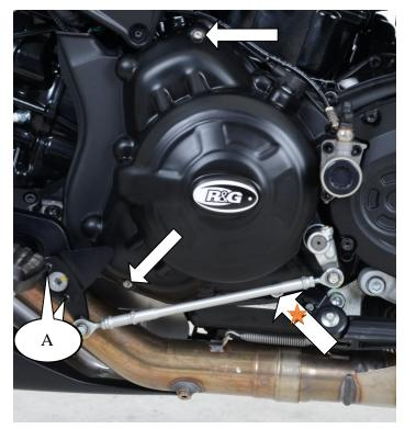
In this kit there should be: 1 x Engine Case Cover (ECC0215). 3 x M6 x 45mm long Button Head Bolts. 1 x M6 washer 3x Spacers (S0820).
